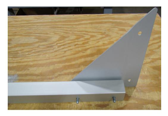
Place opposite paired Bent Upper Gusset on other side of Upper Support. Add Washers to bolts before tightening Nylock Nuts.
