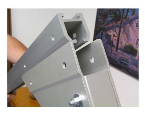
Attach Transverse Beam, with open channel downward, to one Upright Support.
