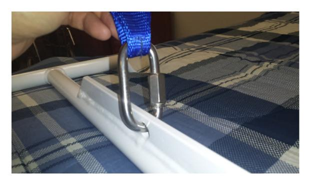
Hand-tighten Link to close completely. Raise Lift Belt and Lift Bar to Motor Housing.
