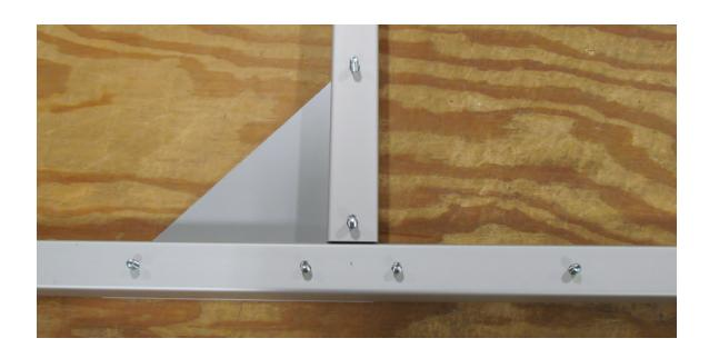
Place Flat Gusset over top of Base Support and Lower Support. Fasten Nylock Nuts on all six bolts. Do not over-tighten. Repeat process for second Lower / Base Support.
