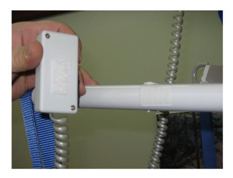
Attach the Remote Control using the Hook & Loop tape included and place in a convenient location. We suggest attaching it to the Lift Bar or Lift Motor.
