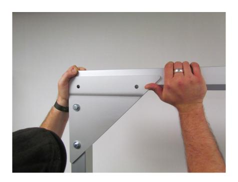
Slide Transverse Beam into opposite Upright Support and attach with two 3 ½" Bolts with Nylock Nuts. Tighten all hardware connecting Beam with Upright Supports. Do not over-tighten.
